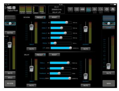
Effect (reverb): It's function is to change the original sound waves, modulate or delay acoustic phase, enhance harmonic properties, etc, to produce a variety of special sound effects. Apply across the sound effect(effects, impacts).
