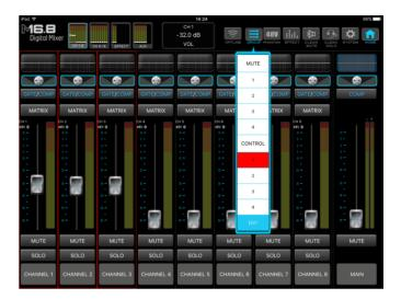
48V:Independently control 16 input channel's 48V phantom power on/off. Which channel requires 48V power supply, you lit the corresponding channel icon on.
