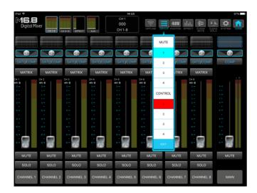
Control group: After entering control edit interface, as picture shows: after click "control 1", select 1,2,3,4 channel, and then select the simultaneous adjustment function that you want, then click control group"1", so that you can adjust the parameters of 1,2,3,4 channel at the same time.
