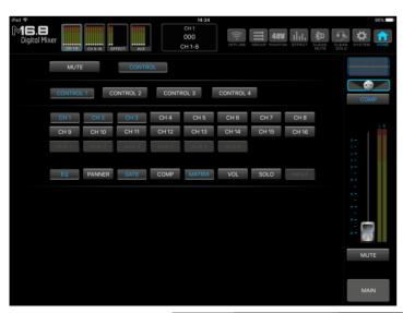
2.PAN: L/R PAN adjustment, adjust the distribution of sound source in space, such as adjust to the left, put the sound source to the left channel.
