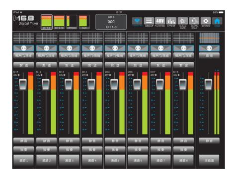
The main interface 1 to 8 input channels and the main output channel, press "CH9-16" to switch to 9-16 channel, press "AUX" switch to the auxiliary output channel.
