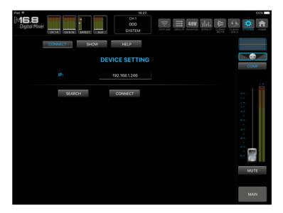
CONNECT: Via searching out the mixer or enter IP manually to connect the target mixer.
